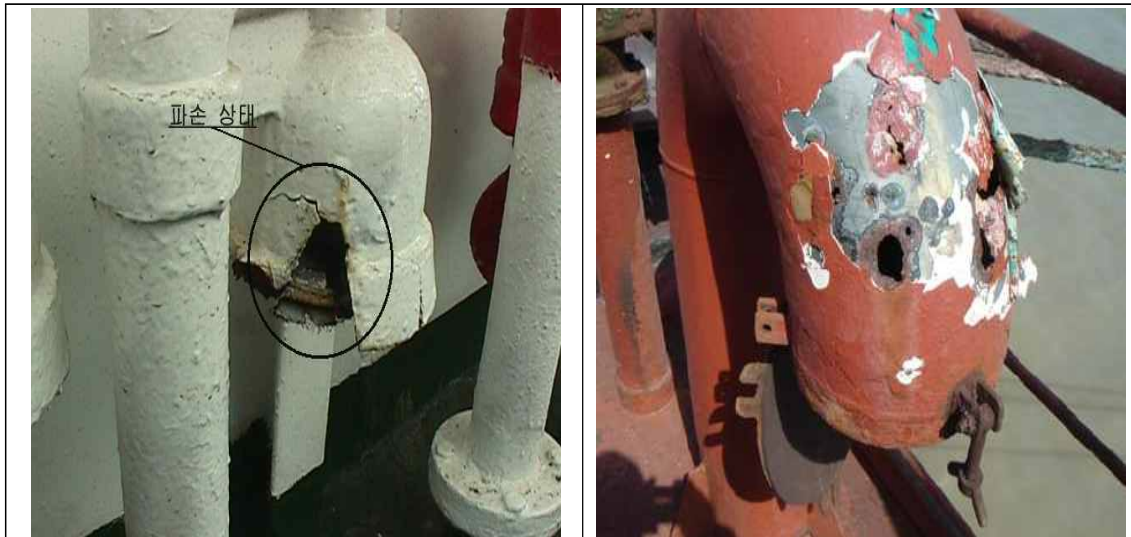
7. External examination of all air pipe heads installed on the exposed decks (Ch 2, 202. 1 (1) (g) of the Rules)
